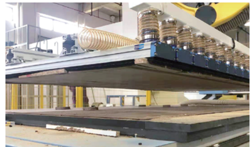
Foam suction HVGP absorbs wood
