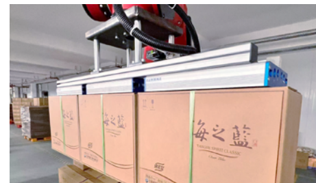
Foam suction HVGP absorbs packaging carton
