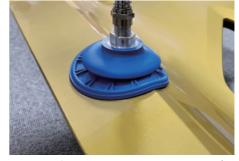
\*HAB suction cups transport concave and convex workpiece surfaces
