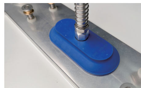
*HAF suction cups carry long workpiece surfaces
